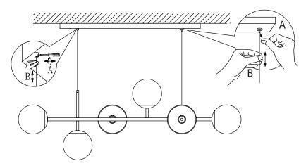
When adjusting the length of the metal wire, please note to press down the button at the canopy before you start pulling the metal wire, in order not to damage the lamp.
